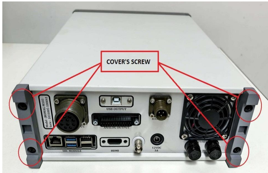
Figure 9. Location of upper and bottom cover screws.
