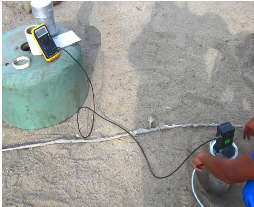
Figure 11. Orientation of the Y component with magnetic north.
