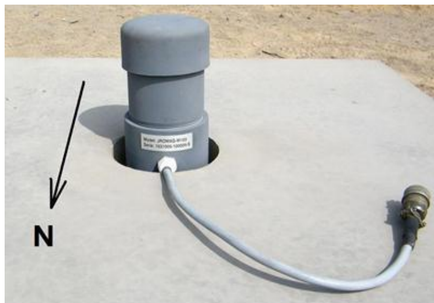
Figure 3. Orientation of the sensor unit for field installation.
