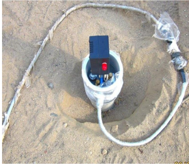
Figure 8. Location of the BNC connector, red cap.
